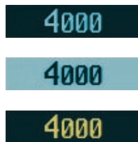
Figure 2-15 Colors Associated with the Altitude Alerter
