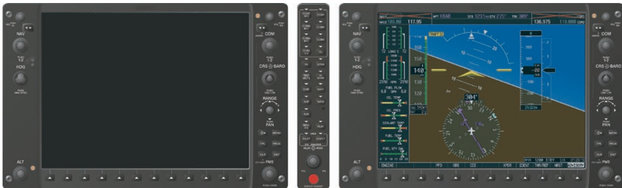
Figure 1-4 G1000 Reversionary Mode: Failed PFD
